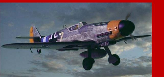
The main German fighters faced by the Tuskegee pilots were the Messerschmitt Me-109 Models "F" and "G". The Me-109G was powered by a 1,475 hp Daimler-Benz engine. It had a range of 435 miles (700 km) and a top speed of 400 miles per hour (640 km). It was armed with one 30mm MG FF cannon firing through the nose and two 13mm MG 131 machine guns firing through the propeller arc and two more 20mm MG151 cannons in the wings.
